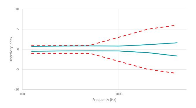
Fig. 9 Directivity according to ISO 3382. Upper and lower curves are the ISO 3382 tolerances
