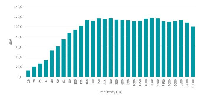
Fig. 4 Sound Power Level Spectrum - 1/3 oct
